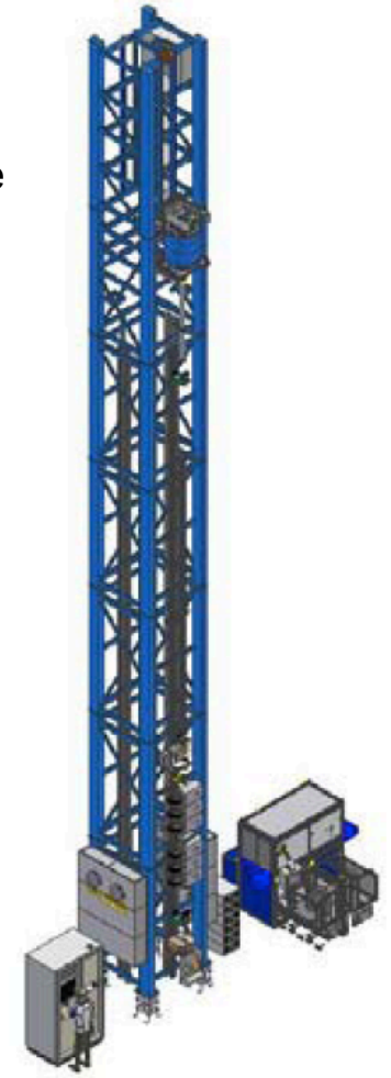
Tall OFC 20 Fiber Draw Tower for mass production of Single-Mode optical fiber
